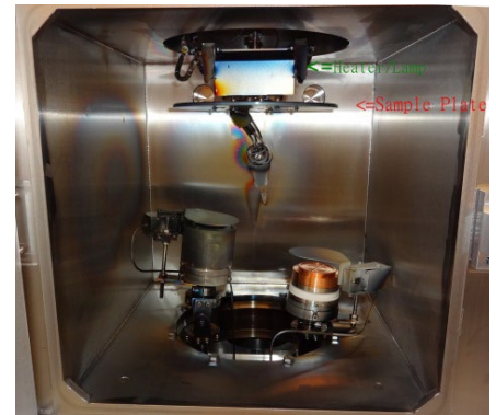
Figure 1 Vacuum chamber with right Torus cap off. (Also w/o required chamber liner)
