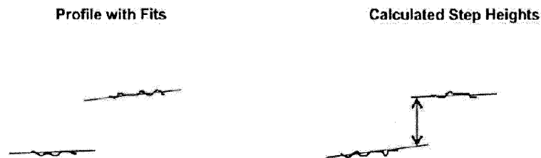
Figure 3-29. Line Fitting for Single-Sided Step Heights
